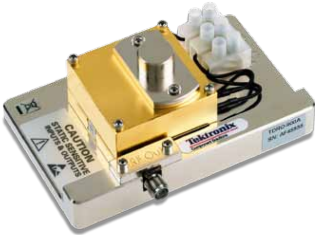
TDRO-900A—Shown in bench configuration, with Optional Base and SMA Connector
